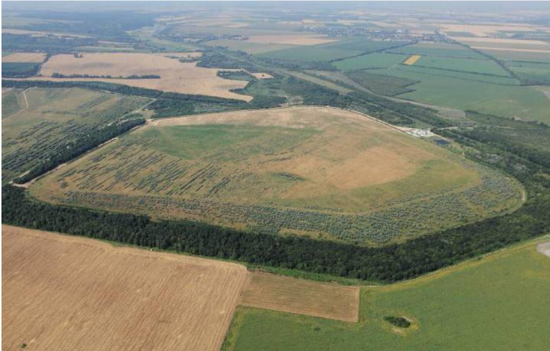
Figure An7. 3-2: Remediated uranium industry tailings pond
