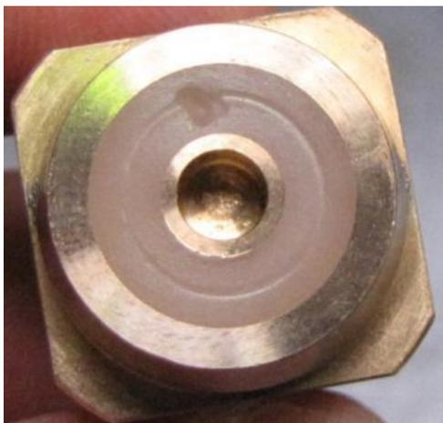
*Surface defect on the reducer's closure element*
