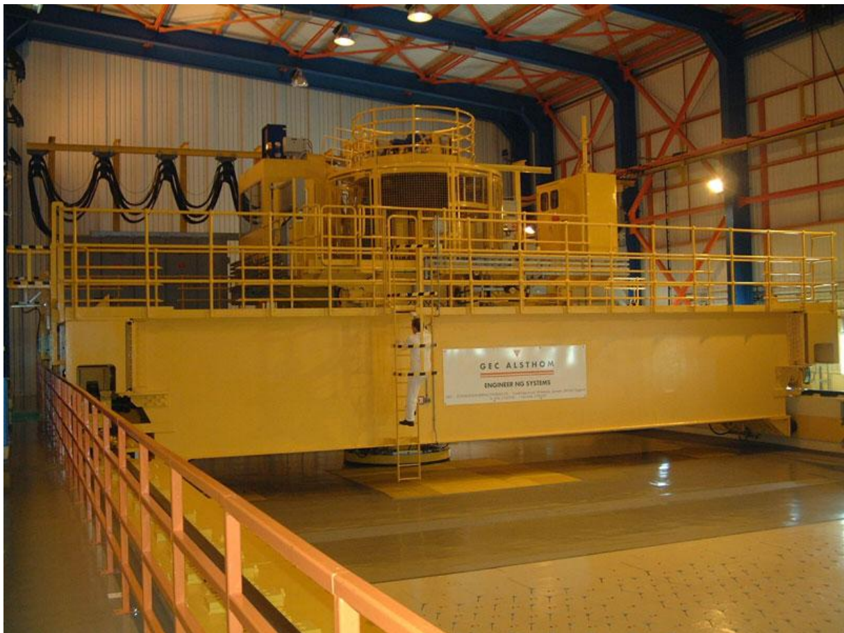
Picture 2.2-1: ISFSF fuel recharge machine (Source: http://www.rhk.hu/letesitmenyeink/kkat/a-kkat-uzemeltetese/ )
