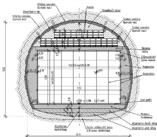
*Formation of the reinforced concrete vault in I-K3 disposal chamber*
