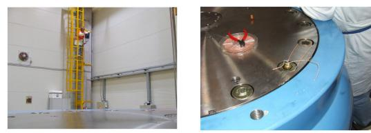
Figure 9. Surveillance of the loading hall with an IAEA camera and sealing of the containers with common seals
