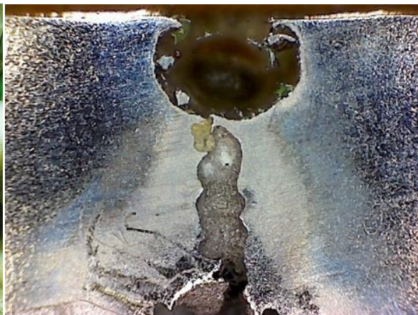
Cross-section of a corrosion pit, cut from the pipeline at Unit 3
