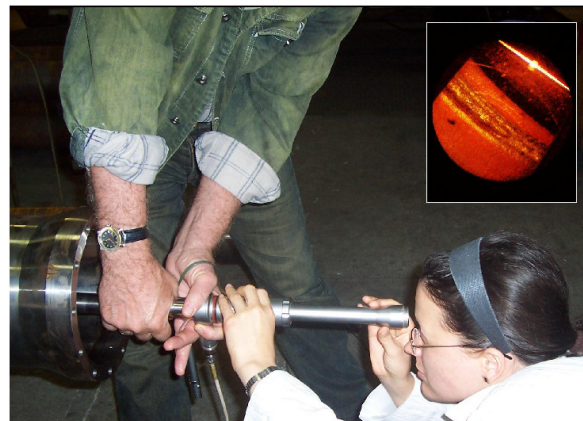
Storage tube internal welding control
