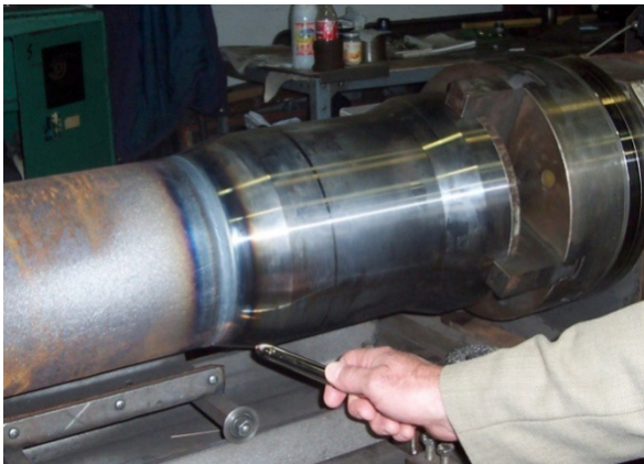
Storage tube external welding control
