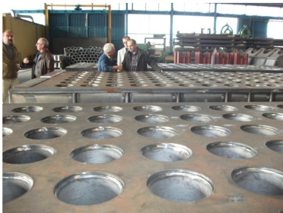
Visual control of charge platform sections before coating
