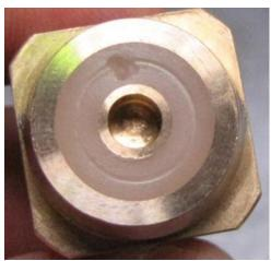
Surface defect on the reducer's closure element
