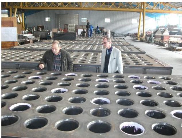
Visual control of charge platform sections
